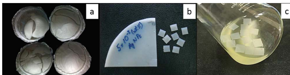
Figure 1. (a) AgNP traps in a round aluminum mold, (b) specimens of a PE/AgNP disc (left side) and PE/AgNP squares for antibacterial testing (right side), and (c) mixed tested bacterial cultures with PE/AgNP nanocomposites. [Color figure can be viewed in the online issue, which is available at wileyonlinelibrary.com .]
